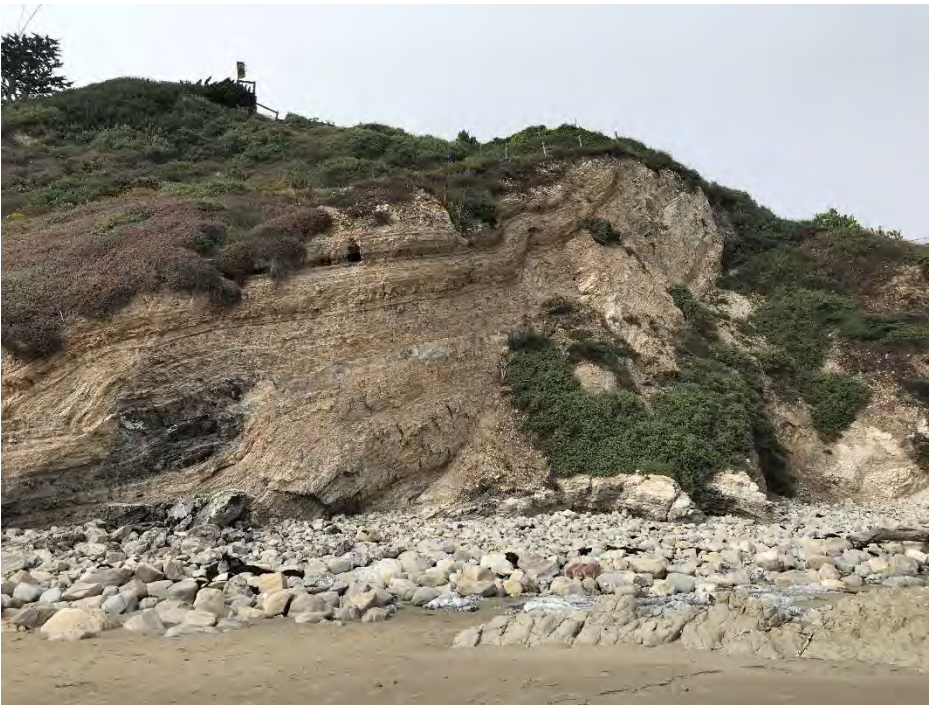
- Daylighted Monterey Shale Bedding on East Side of El Camino de la Luz Landslide (near CoSMoS Transect 4000)
