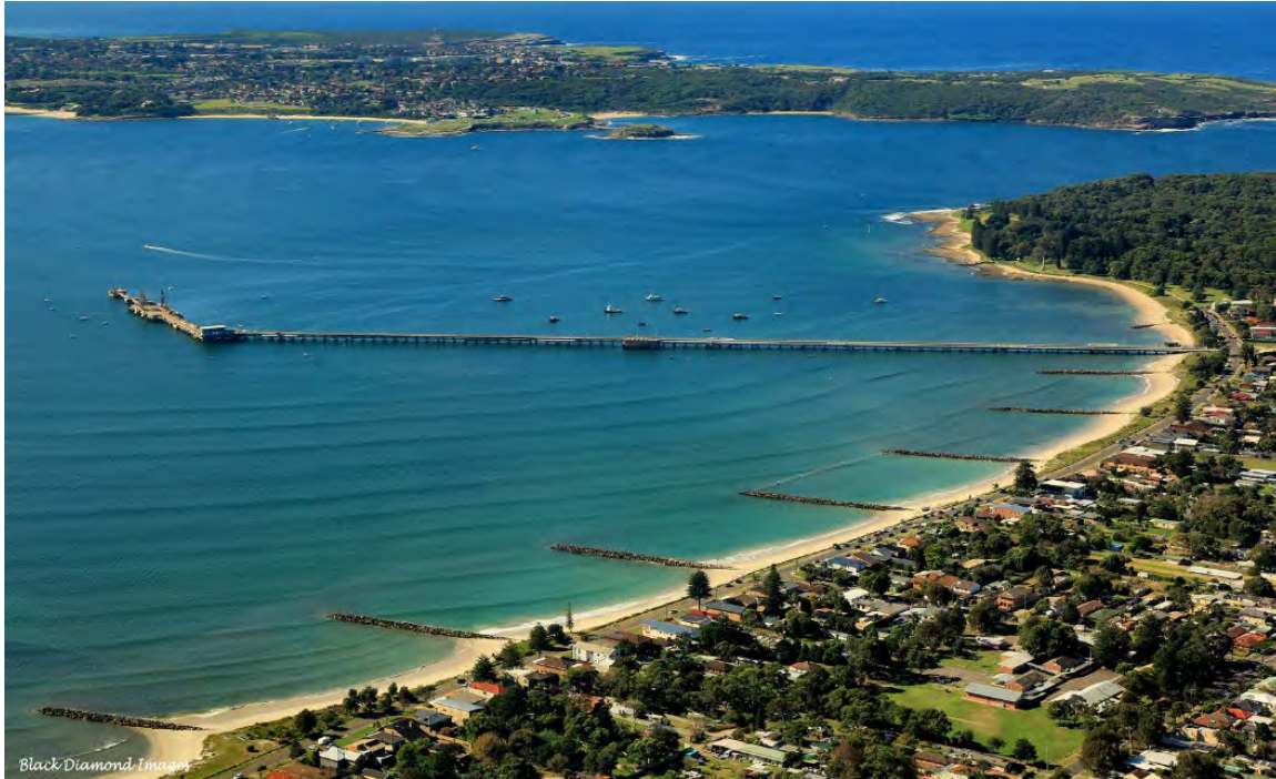
Figure 5-3 Photo of a series of groins in Sydney, AUS
