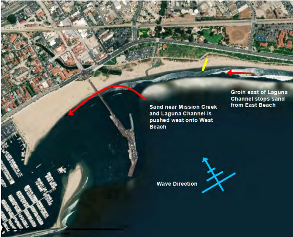
Figure 7-5 Example of groin and sand movement during south swell
