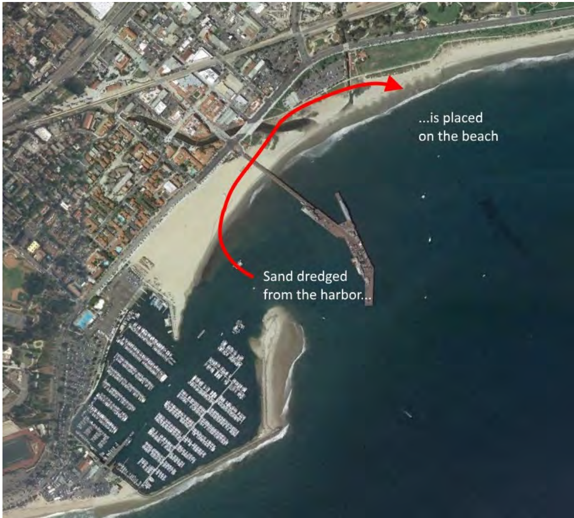
Figure 7-4 Sand bypassing concept
