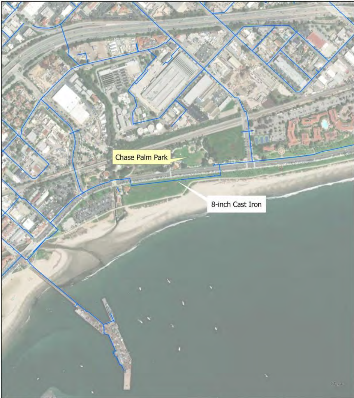
Figure 7-3. Near-Shore Potable Water Distribution Pipelines
