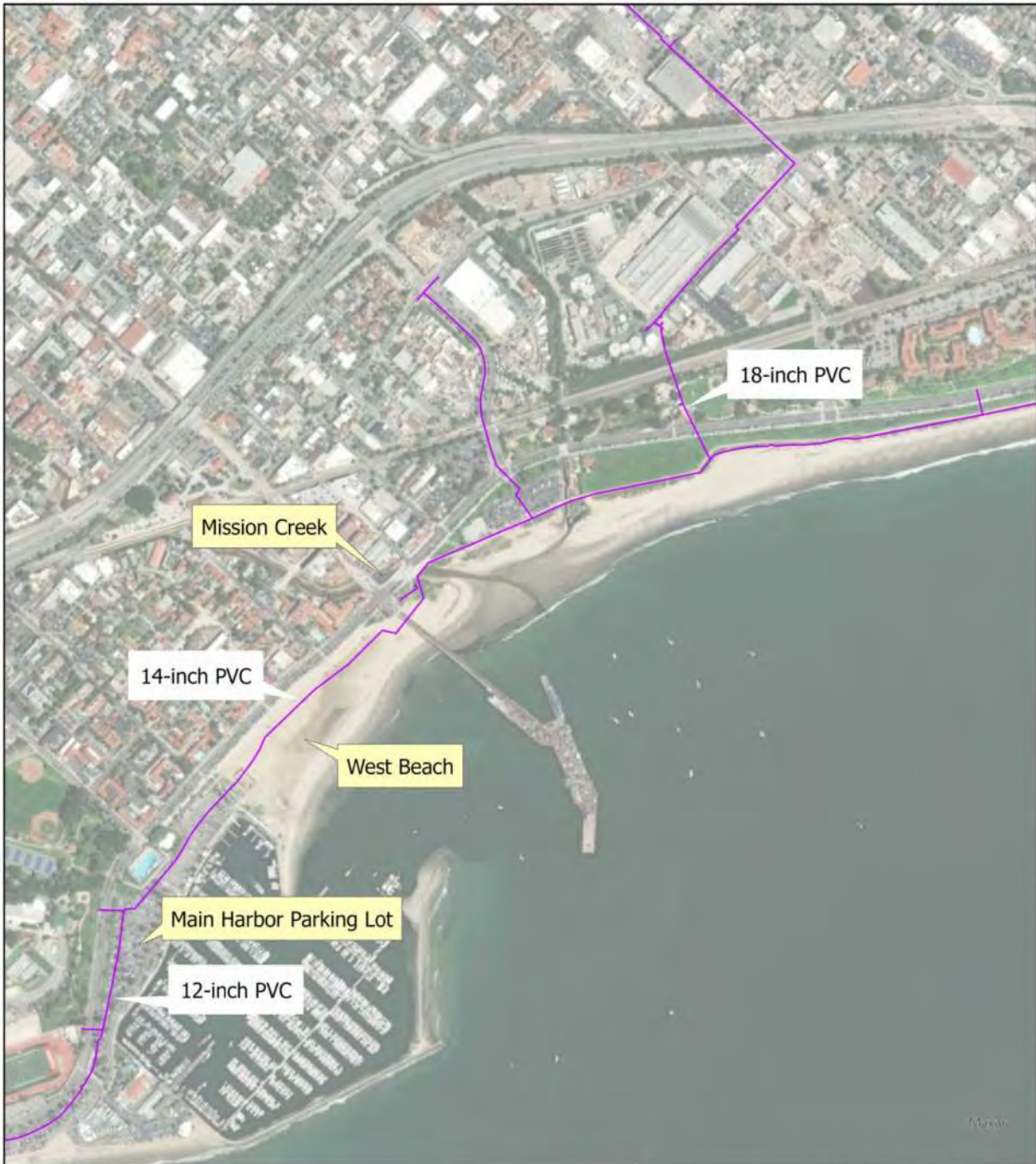
Figure 8-3. Recycled Water Distribution System in Coastal Area
