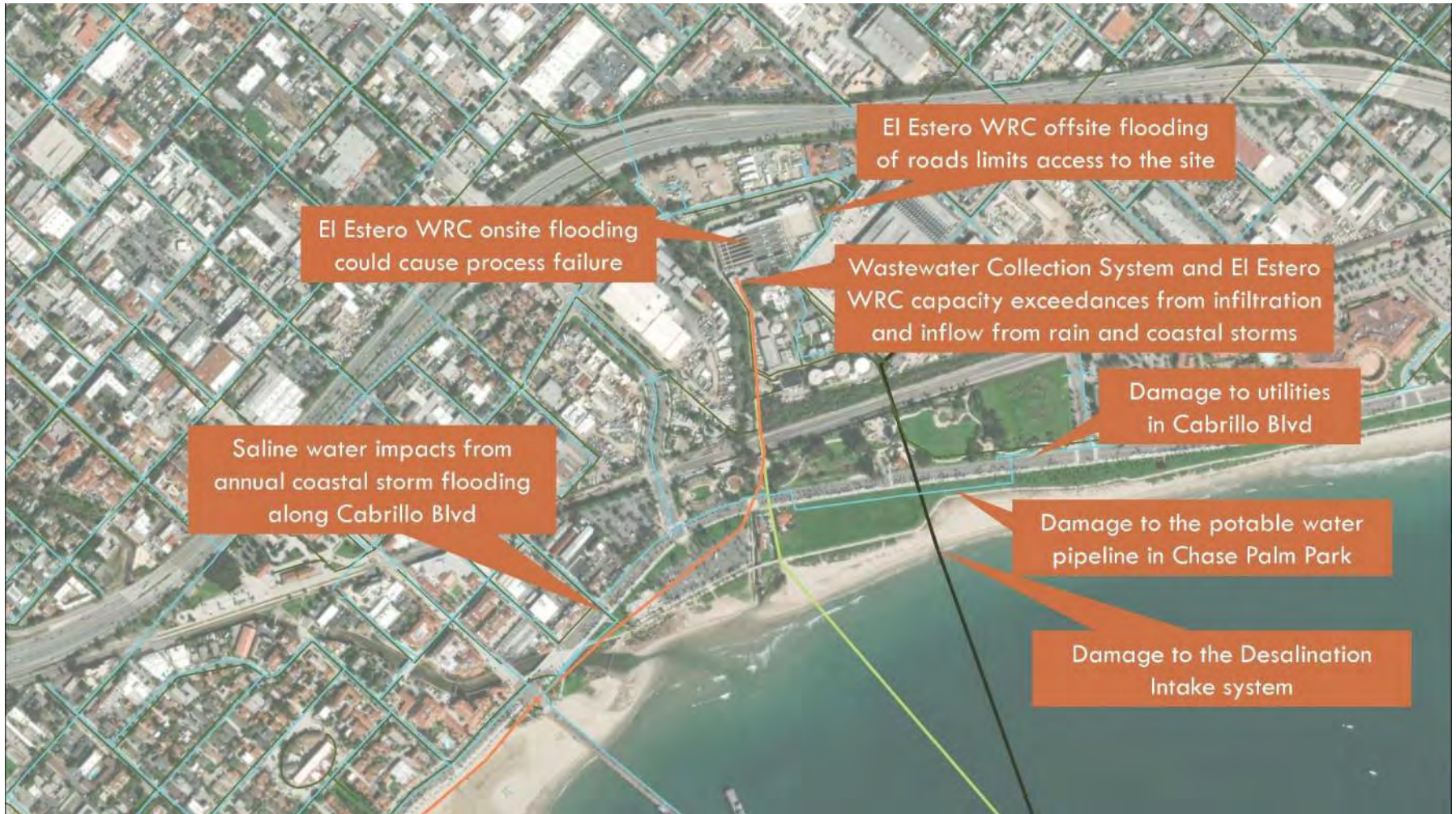
Figure ES-5. Highest Near-Term (Next 25 Years) and Mid-Term (25 to 50 Years) Infrastructure Risks from Climate Change
