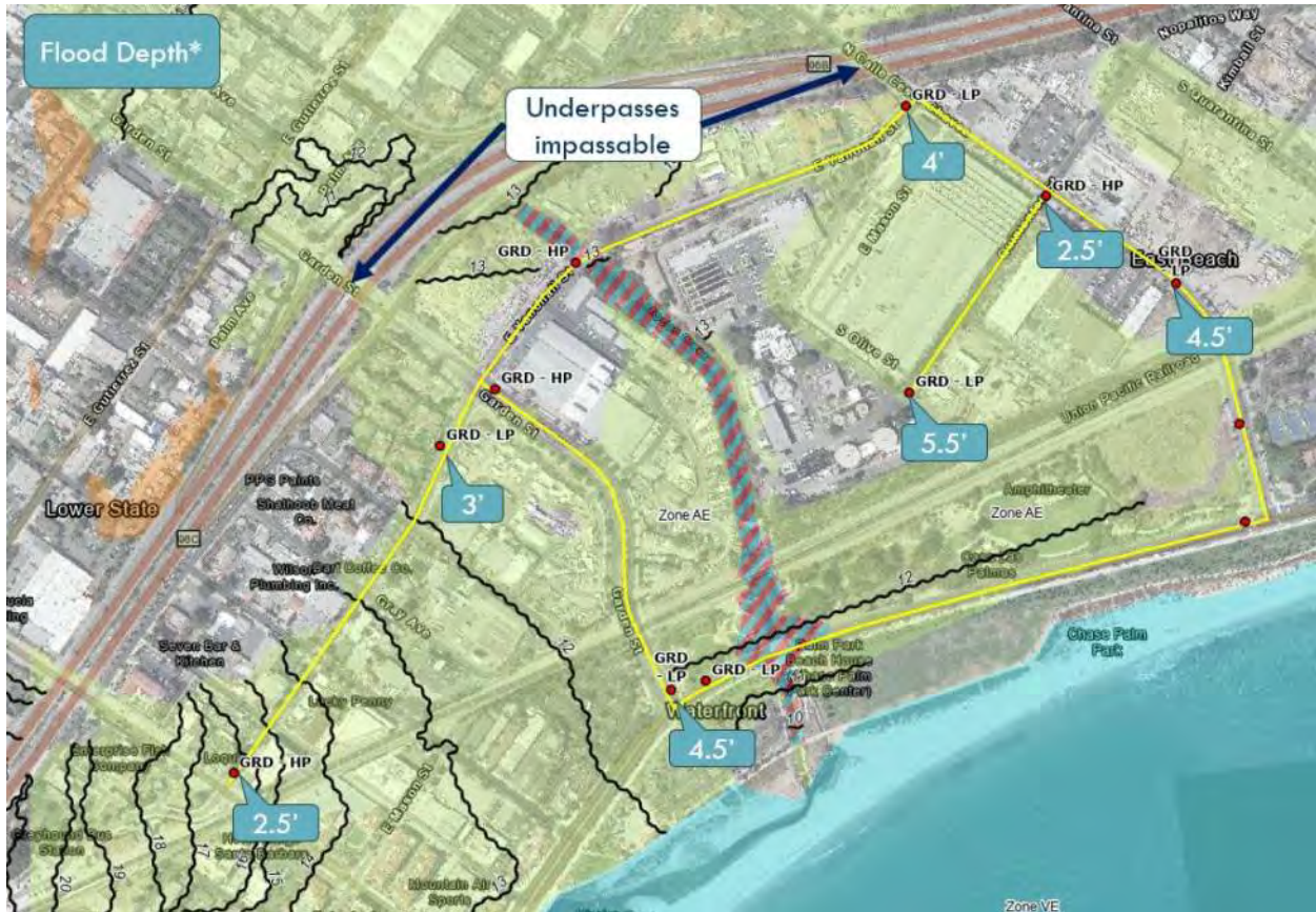
Figure Note: This figure shows the extent of the historical FEMA 100-year flood (light green shading) and flood depth at selected road access points to the El Estero WRC area.
