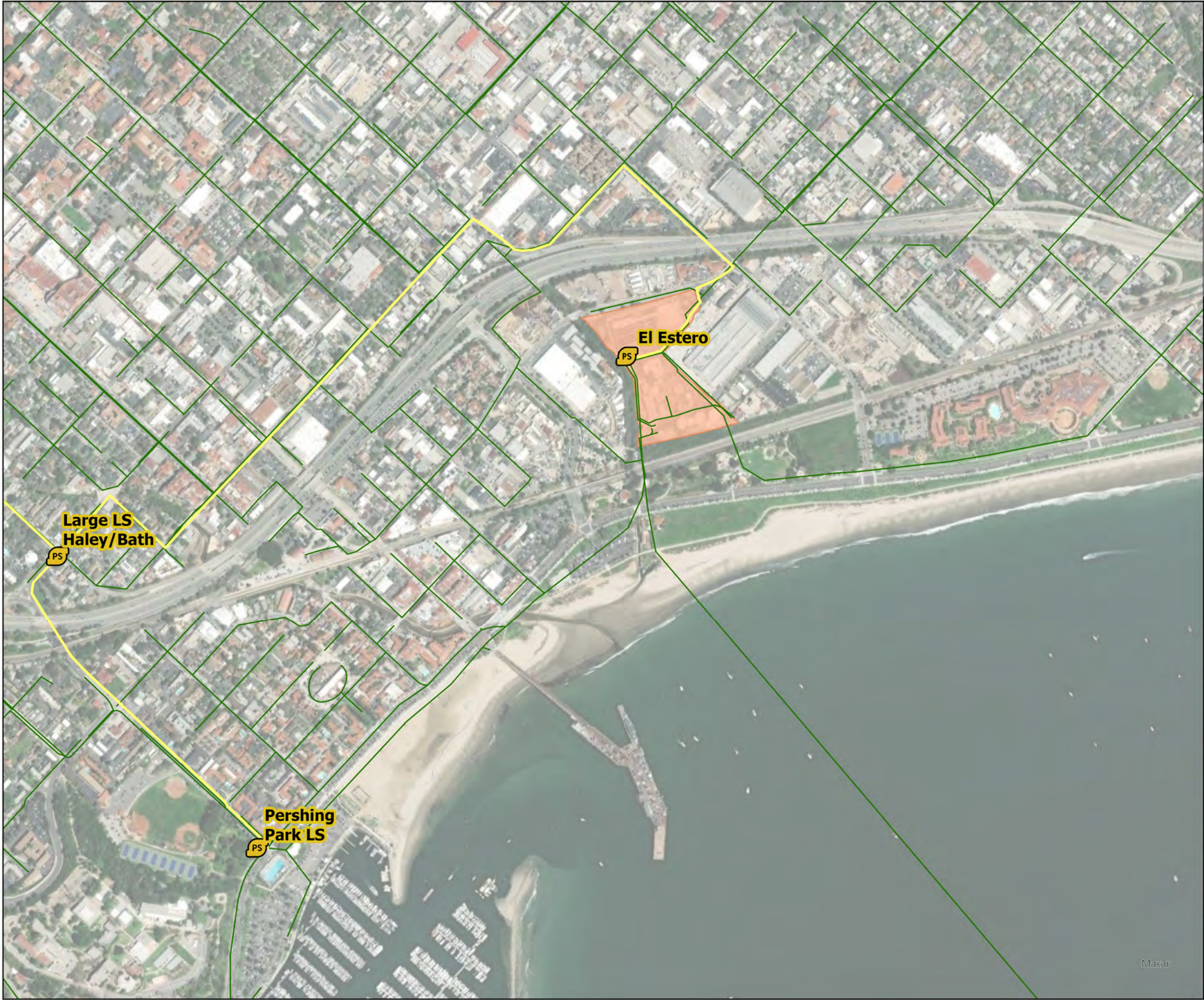
Figure 4. Proposed Lift Stations and Force Mains for El Estero WRC Relocation
