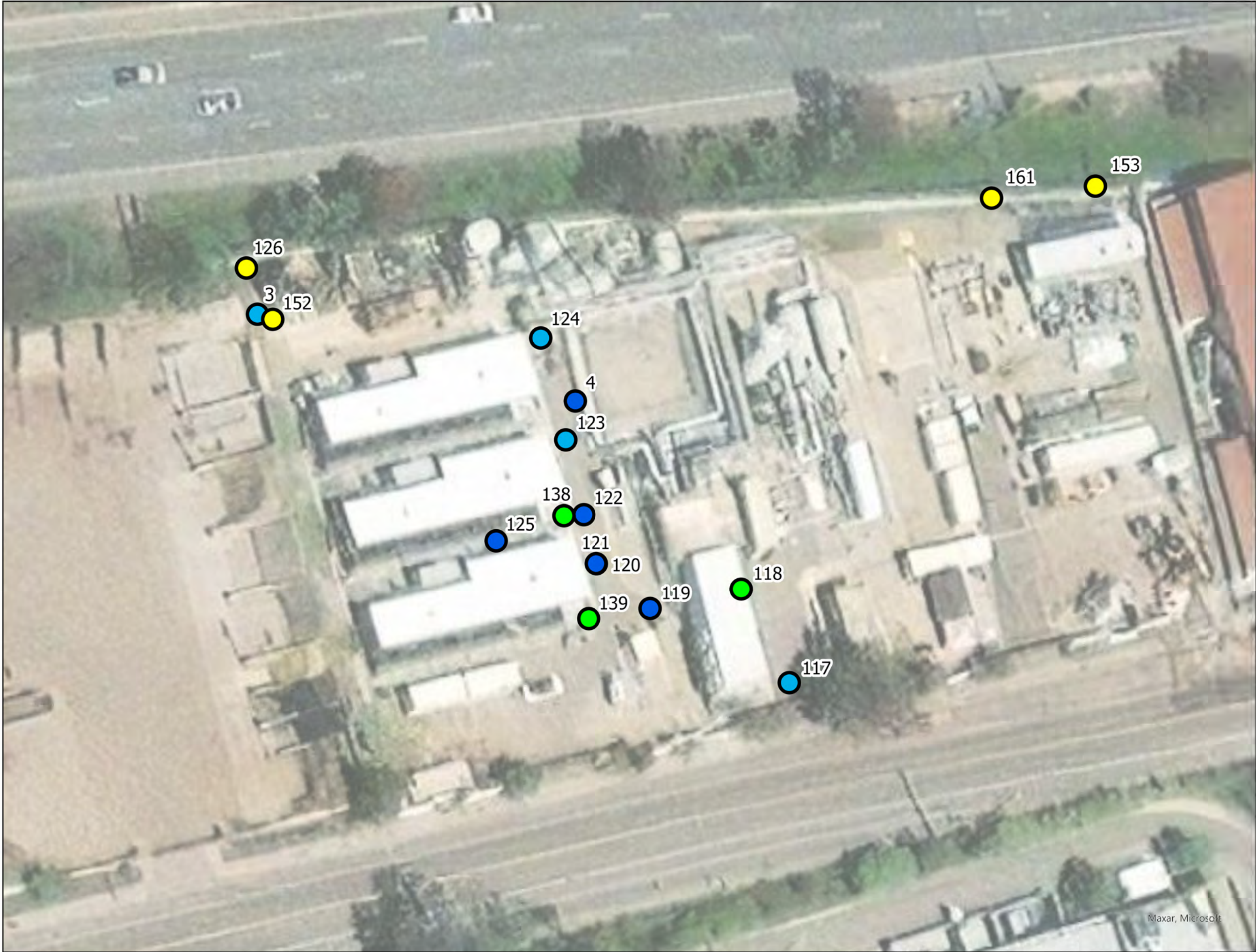
Figure 6-3. Desal Plant Survey Points Measured Compared to Historical FEMA 100-yr Flood Depth
