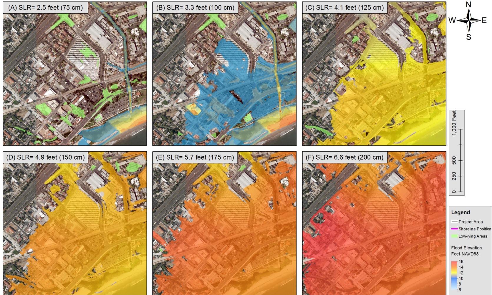
Figure 10: 100-year Coastal Storm Flood Hazard Map at Existing Grade
