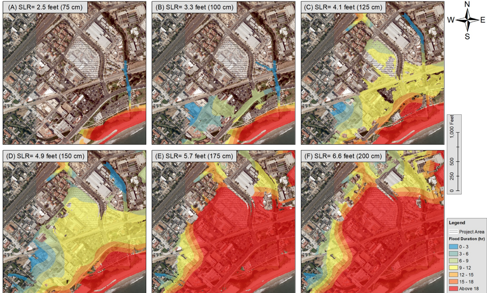
Figure 11: Annual Coastal Storm Flood Duration Map at Existing Grade
