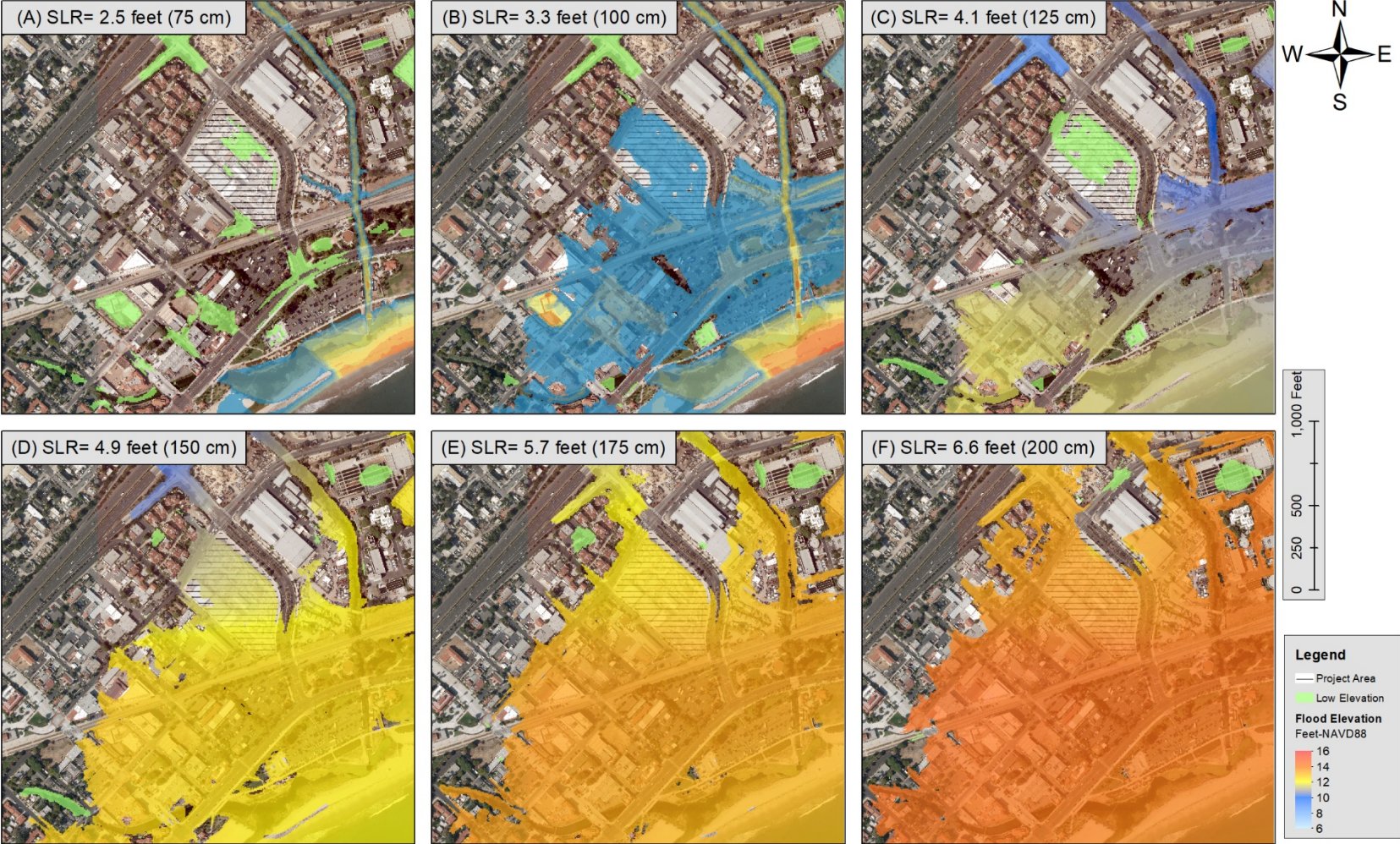
Figure 9: 20-year Coastal Storm Flood Hazard Map at Existing Grade
