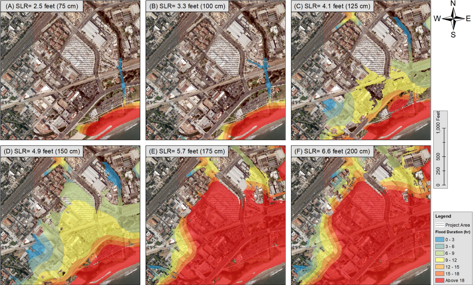
Figure 12: 20-year Coastal Storm Flood Duration Map at Existing Grade
